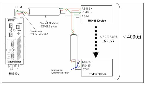
Figure 12: Conceptual recommended RS485 wiring diagram
